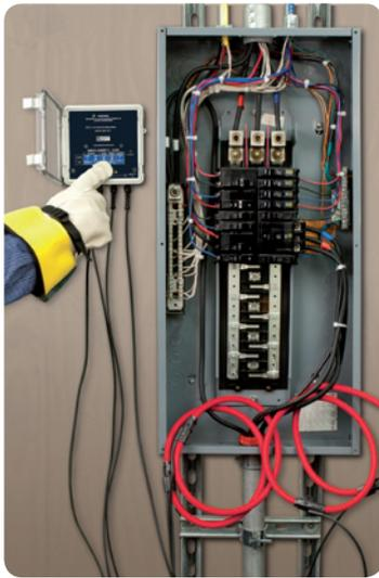
The ML 914 and AL 834 Simple Logger® II models are 4-channel TRMS AC current loggers.
