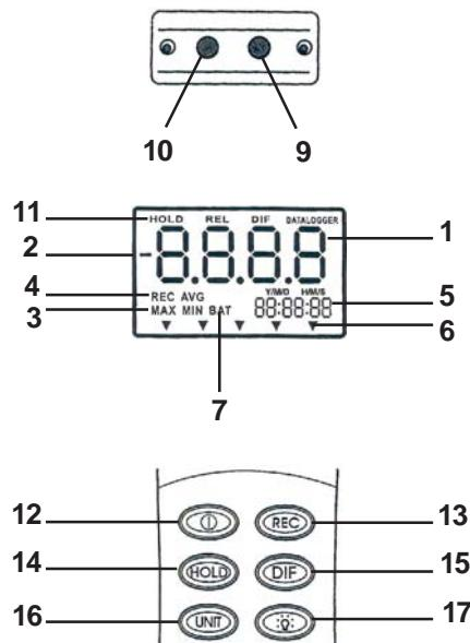
1. Main screen indicating the pressure measurement in the unit selected
